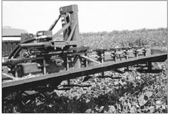
The “weed topper” was designed to mow weeds that rise above the soybean canopy, greatly reducing bean-staining problems at harvest.
