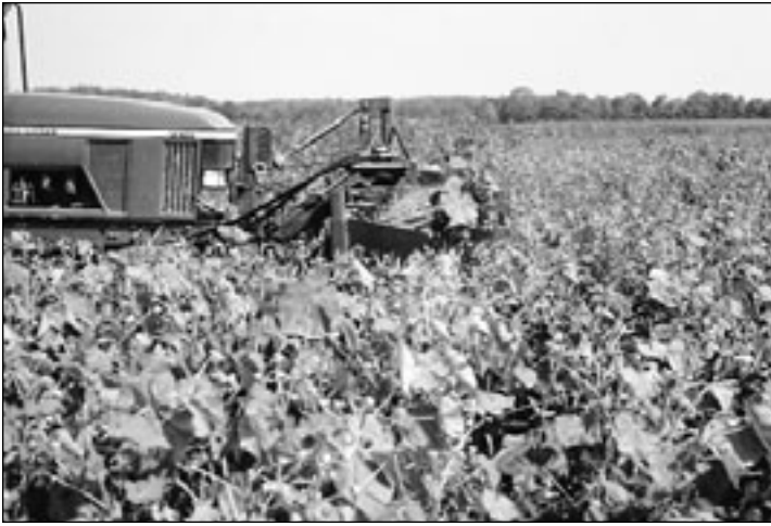
The “weed topper” was designed to mow weeds that rise above the soybean canopy, greatly reducing bean-staining problems at harvest.
