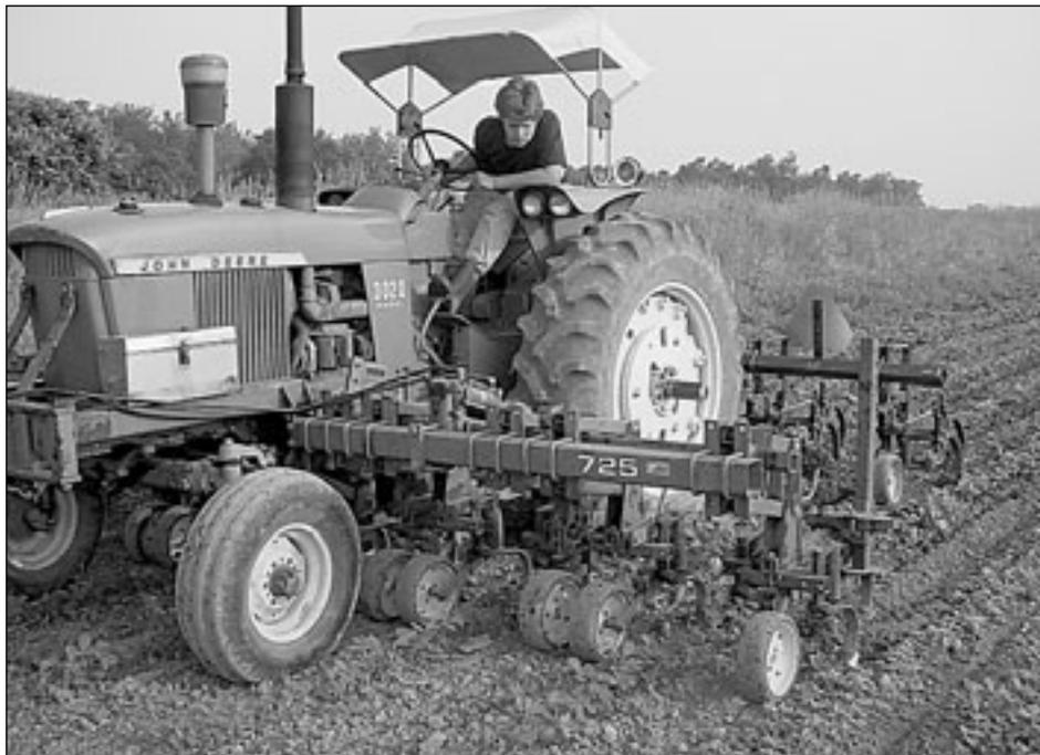
*Peter Martens, cultivating soybeans on a John Deere 3020 with JD725 front-mount cultivator and a IH133 rear-mount cultivator; both with C-shank teeth. The front has half sweeps, the back has sweeps. The front cultivator is modified to have two gangs per row instead of the standard single gang in the middle of the row. The rear cultivator is modified with a side shifter to keep it aligned with the front cultivator on side hills.*
