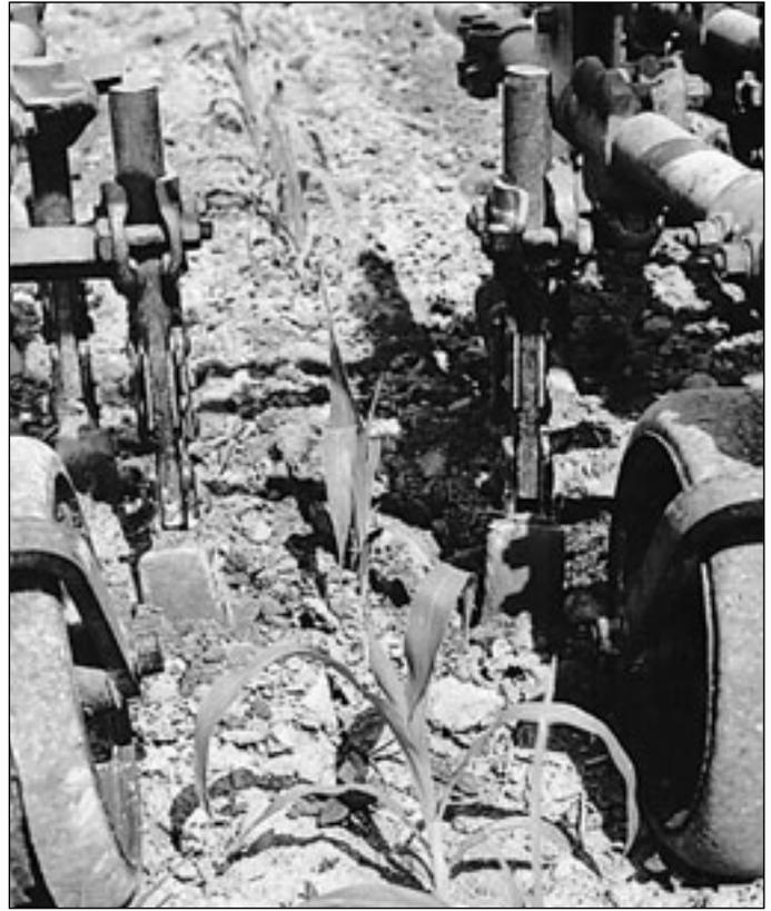
*Front and rear view (before and after) of an older-style John Deere trip-shank cultivator. It is equipped with small shovels that allow the operator to cultivate very small crops at higher speed. This runs relatively shallow. This configuration is suitable for small weeds but not aggressive enough for large weeds or high weed populations.*
